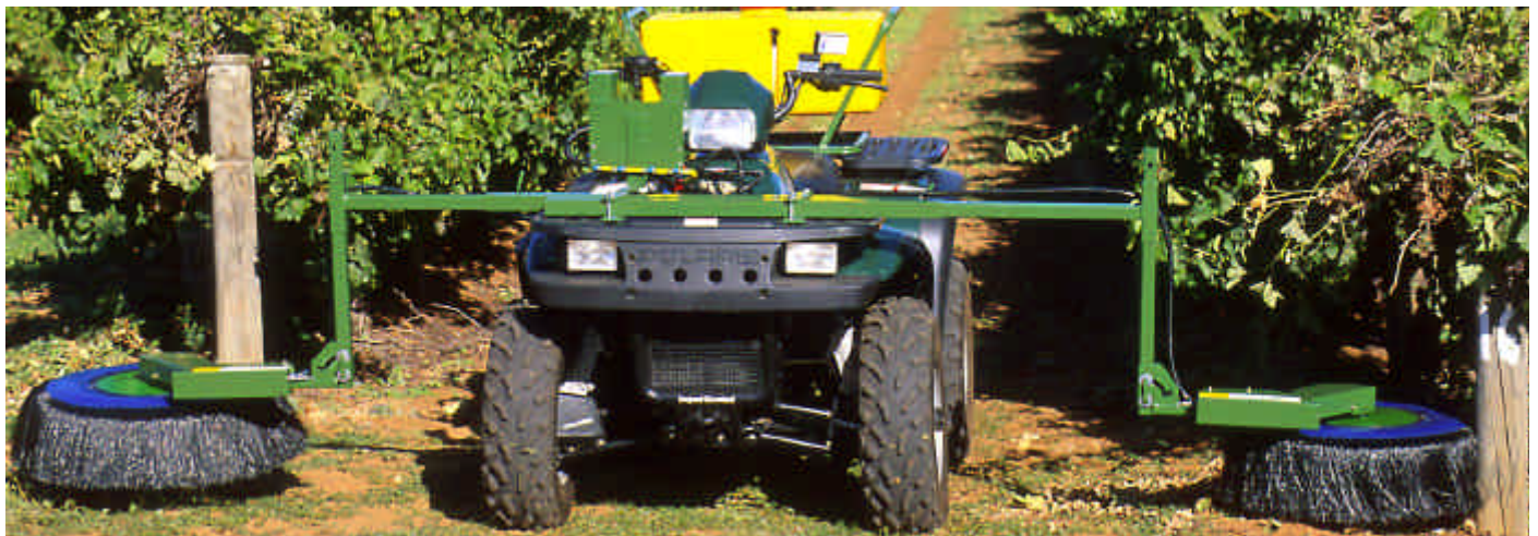
Typical Circular Sprayer Vineyard Setup
